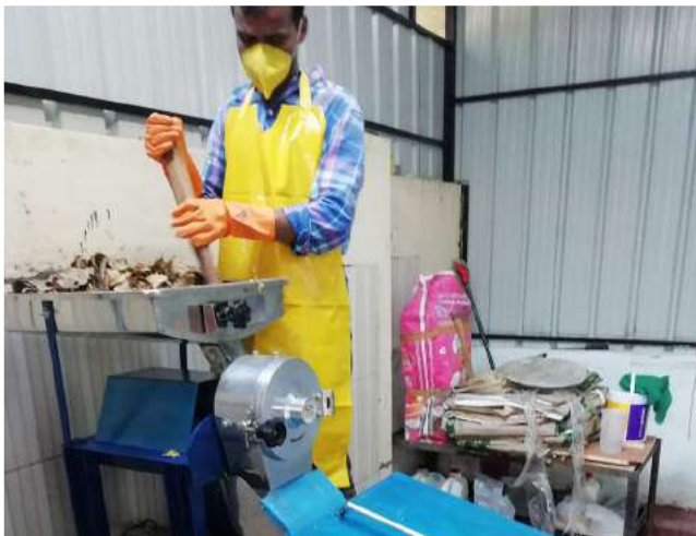
‘Suchitha,’ the food waste to manure converter
